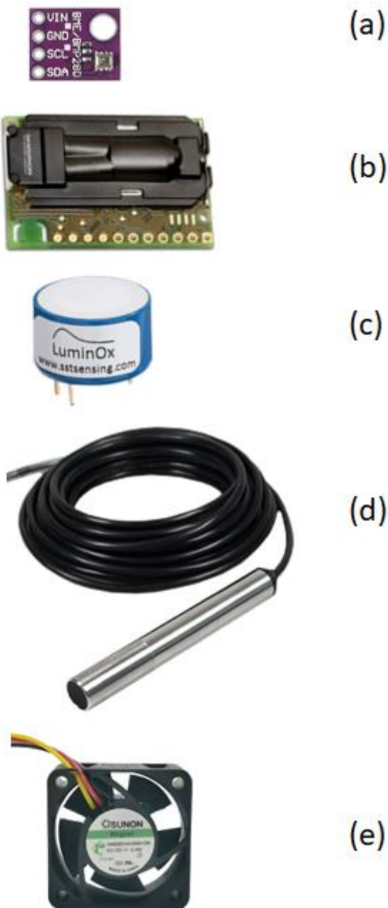
155 Figure 6. Used sensors and fan: a) BME280, (P, T, and RH), b) SCD30 (CO 2 ), LuminOx (O 2 ), d) OXYBase (O 2 ), e) Maglev fan.
