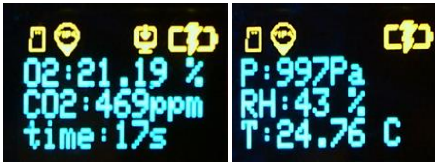
Figure 2. small 0.96", yet very readable, OLED display permuting screens with different useful information.
