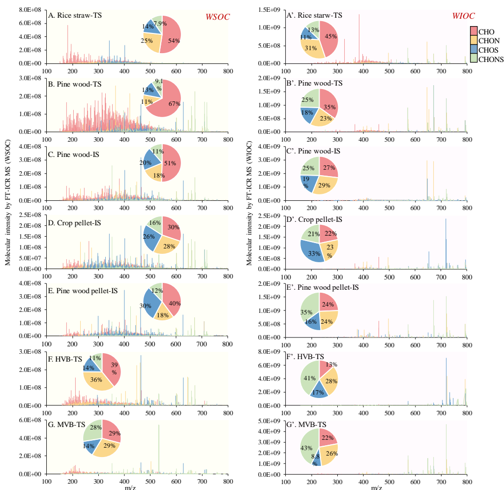
245 Fig. 2 Negative ESI FT-ICR mass spectra of WSOC (A-G) and WIOC (A'-G') from the seven 246 aerosol samples, TS represents combustion in the traditional stove and IS represents combustion in 247 the improved stove. Different formula groups were color-coded. The pie charts showed the relative 248 intensities of different formula groups.
