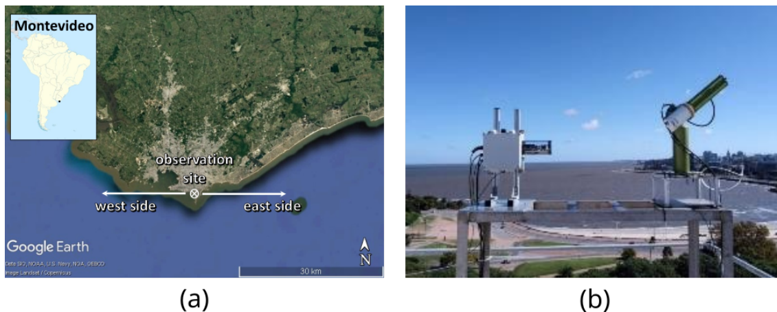
Figure 1. (a) Map of Montevideo and the geometry used for the MAX-DOAS measurements. The observation site is located at the Faculty of Engineering. The spectrometer scans a vertical plane from east to west at several elevations. (b) Picture of the MAX-DOAS instrument (left) and the CIMEL sun photometer (right) on the roof of the building.
