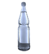
165 Figure 1: The reusable glass pool bottle. Two rings (in the middle and at the bottom) function as "shock absorbers" to prevent breakage in the filling and cleaning process. The pearl-like patterns at the bottle neck expresses freshness while enabling a good grip (Bielenstein, 2019).
