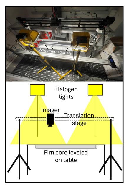
**Figure 2.** Top: Photograph showing the laboratory setup. Bottom: diagram of the laboratory setup. The imager was mounted on the translation scanning stage that moves linearly along the firn core segment. The core is illuminated by halogen lamps to provide broadband radiation. Spectralon panels were placed along the side of the firn core to convert measured radiance to reflectance.
