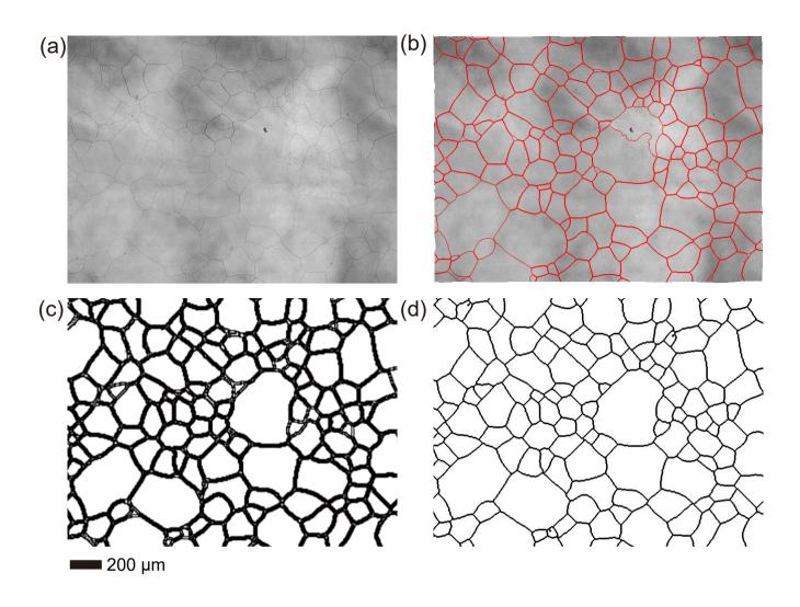
**Figure A2.** Identification, correction and refinement of grain boundaries. (a) The input image. (b) Visualized grain boundaries overlaid on the input image. (c) Grain boundaries subsequent to manual correction and conversion to a binary format. Note that the curvy "grain boundary" in the large grain in the center of the image was manually removed. (d) Refined grain boundaries with a maximum width of two pixels.
