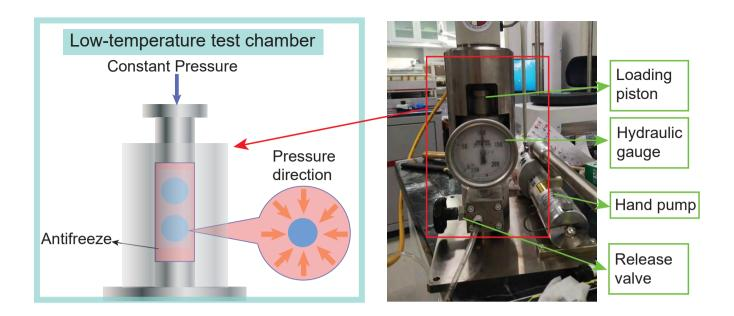
**Figure 1.** Photo and drawing for the cold isostatic press (CIP). On the right is a photo showing CIP under a pressure of 100 MPa. On the left is a drawing of the pressure vessel in the low-temperature test chamber, which samples inside. Antifreeze, acting as the pressure medium, delivers hydrostatic pressure on the samples.
