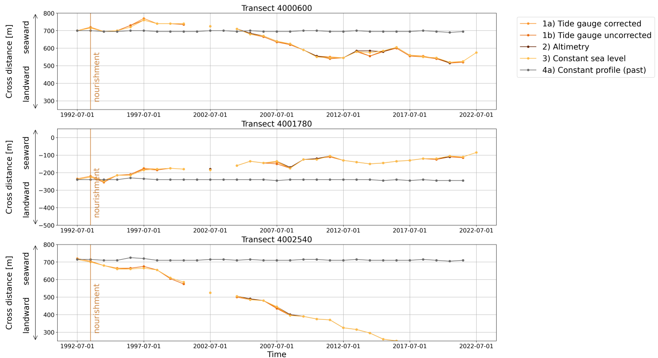
Figure 6. Three examples of cross-shore timeseries for the transects indicated in Fig. 5 showing landward trends in West and East Ter-schelling, and seaward trends for the central coast. The cross-distance on the y-axis is defined to point landward in the negative direction, while more positive values indicate a movement seawards. A negative trend therefore can be interpreted as a retreating shoreline, whereas a positive trend indicates an advancing shoreline. The absolute values depend on the definition of the coordinate system along the transects and can not be compared.
