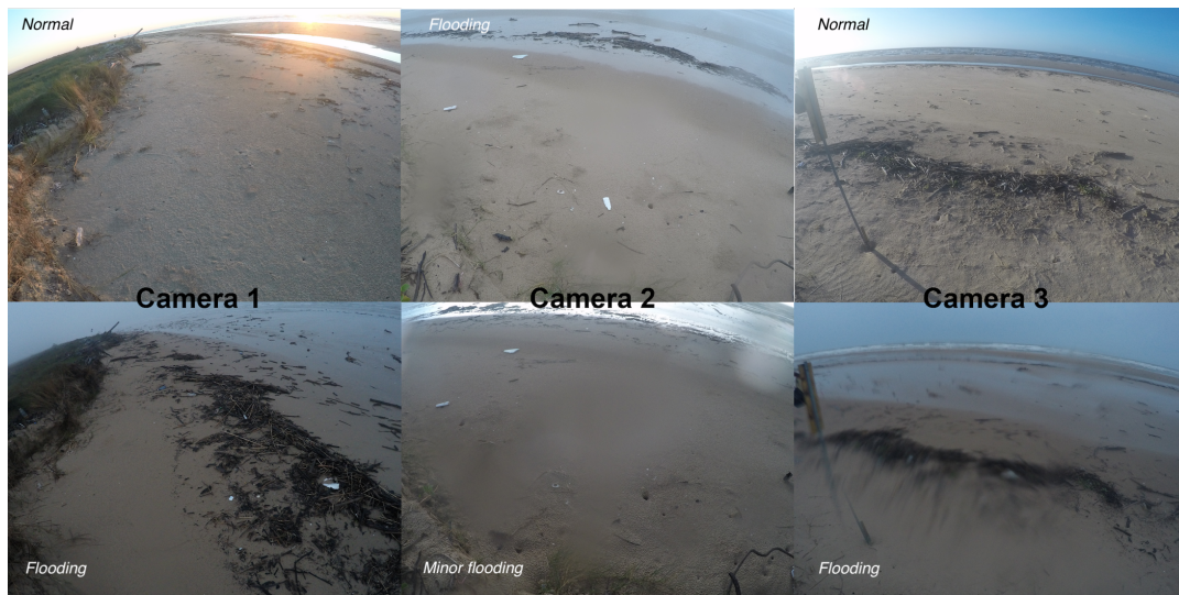
Figure 2. Contrasting images captured from our three cameras depicting both flooding and normal conditions.
