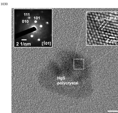
Figure 4: High-resolution TEM image of a 20 nm small poly-cristalline HgS (cinnabar) particle. Inset left) corresponding convergent beam electron diffraction (CBED) pattern. Inset right) Invers Fast Fourier Transformed (IFFT) image from the area indicated by the square.
