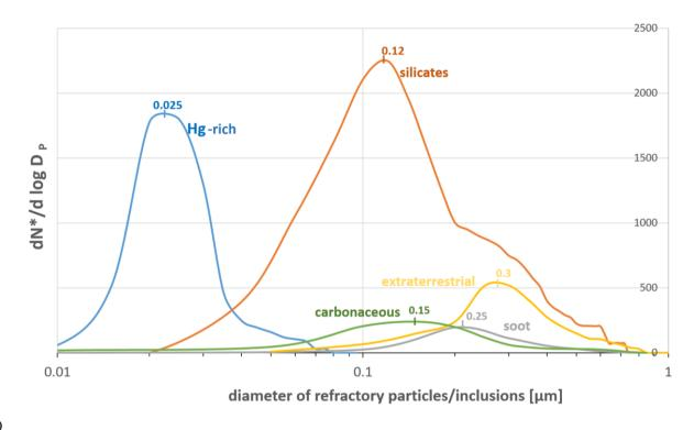
Figure 3: Smoothed relative size distribution of 5 refractory particle/inclusion groups (dN\* = total number of analyzed refractory 1020 particles/inclusions of specific group within all 17 analyzed samples.).
