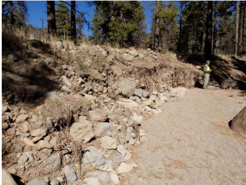
Figure 2. Surveyors performing a BEHI analysis on a typical channel along Spruce Wash. Photo taken in fall 2021 approximately 500 m upstream of Mount Elden Estates.
