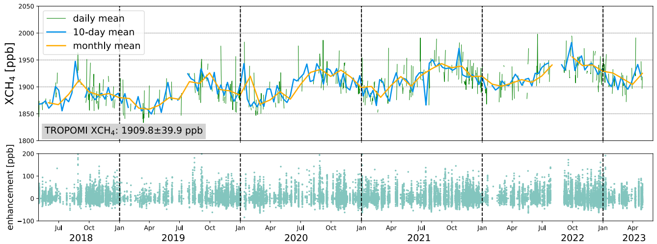
Figure 4: Time-series of average TROPOMI XCH 4 (upper panel) and corresponding enhancement after removing the background (lower panel) over Changzhi region (35.8°N—37.2°N, 112.6°E—113.6°E) from May 2018 to April 2023.
