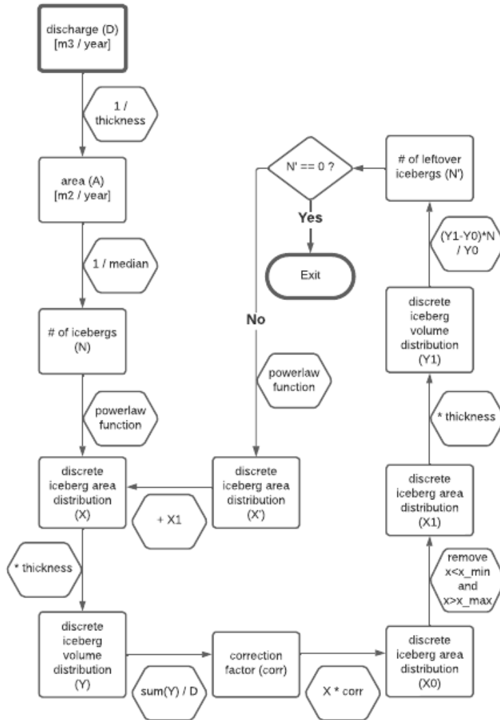
Figure A1. Scheme for the generation of discrete icebergs. The discharge field is integrated to receive a total discharge flux ( D ) which is divided by a reference iceberg height of 250 m to receive an iceberg area flux ( A ). A reference iceberg area size, here the median of the power-law distribution, is used to derive the number of icebergs to be generated ( N ). The median is given by 2^{1/(k-1)}x_{\min} where k is -3/2 and x_{\min} is 0.01 \text{ km}^2 . The number of icebergs N and the minimum area size x_{\min} are used with the Python power-law package to generate N discrete model icebergs with area size X . To compare the generated iceberg volume ( Y ) with the prescribed total discharge, X is multiplied by the reference ice thickness and summed up, to derive a scaling factor ( \text{corr} ). X is scaled with this factor to calculate a discrete area size distribution ( X_0 ) that is consistent with the prescribed total discharge. Those icebergs with areas smaller x_{\min} or larger x_{\max} are removed. For the total amount of removed iceberg volume, a new number of icebergs to be generated is calculated ( N' ). If this is zero, no further model icebergs are needed, i.e. the calculated model icebergs sum up to the given total discharge. If N' does not equal zero, an iterative process is started, in which new model icebergs from a power-law distribution a generated until N' is zero.
