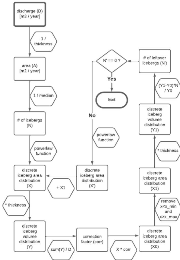
Figure A1. Scheme for the generation of discrete icebergs. The discharge field is integrated to receive a total discharge flux (D) which is divided by a reference iceberg height of 250 m to receive an iceberg area flux (A). A reference iceberg area size, here the median of the power-law distribution, is used to derive the number of icebergs to be generated (N). The median is given by 2^{1/(k-1)}x_{min} , where k is -3/2 and x_{min} is 0.01 \text{ km}^2 . The number of icebergs N and the minimum area size x_{min} are used with the Python power-law package to generate N discrete model icebergs with area size X. To compare the generated iceberg volume (Y) with the prescribed total discharge, X is multiplied by the reference ice thickness and summed up, to derive a scaling factor (corr). X is scaled with this factor to calculate a discrete area size distribution (X0) that is consistent with the prescribed total discharge. Those icebergs with areas smaller x_{min} or larger x_{max} are removed. For the total amount of removed iceberg volume, a new number of icebergs to be generated is calculated (N'). If this is zero, no further model icebergs are needed, i.e. the calculated model icebergs sum up to the given total discharge. If N' does not equal zero, an iterative process is started, in which new model icebergs from a power-law distribution a generated until N' is zero.
