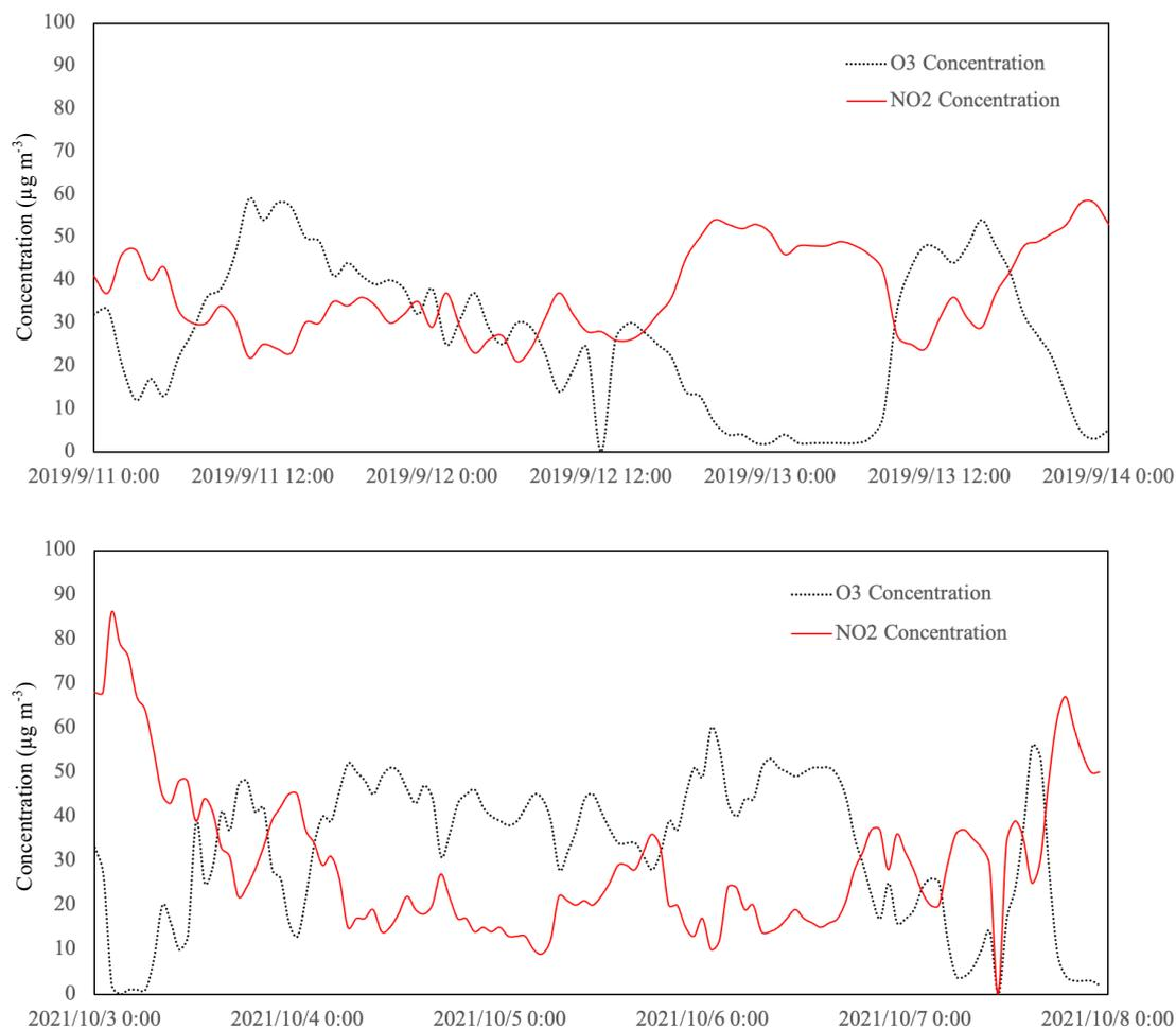
**Response Figure 2.** Time series of hourly concentration of O<sub>3</sub> and NO<sub>2</sub> from ambient air quality monitoring stations near an iron and steel factory in Taiyuan City.
