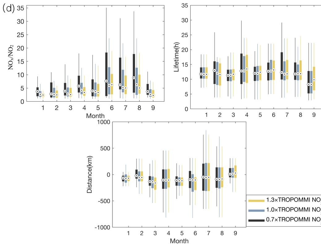
**Response Figure 1.** Different TROPOMI NO<sub>2</sub> for emission calculation based on CEMS using MFIEF: (a) 70%, 100%, 130% cases calculated emission and their uncertainty; (b) the differences between 70% to 100% case and 130% to 100% case; (c) time series of 70%, 100%, 130% cases and their differences; (d)  $\alpha_1$ ,  $\alpha_2$ , and  $\alpha_3$  in each case.
