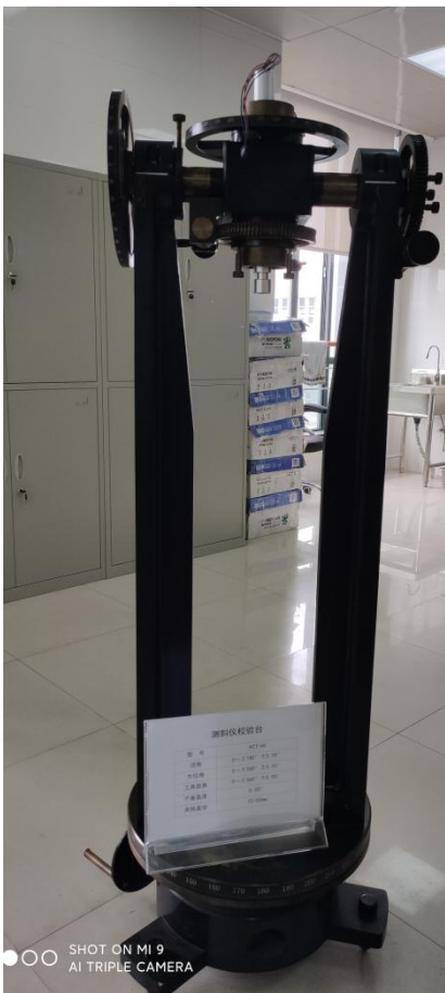
185 Figure 8: HZT-60 inclinometer calibration table.
