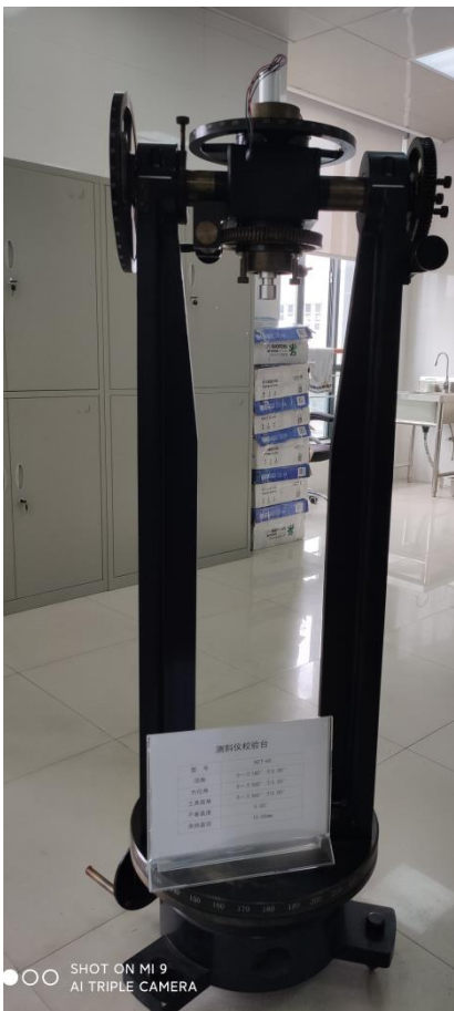
Figure 8: HZT-60 inclinometer calibration table.
