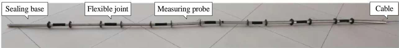
Figure 2: Schematic diagram of continuous full-hole inclinometer probe configuration.
