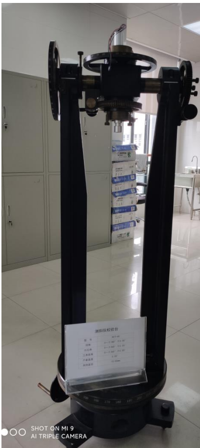
Figure 8: HZT-60 inclinometer calibration table.
