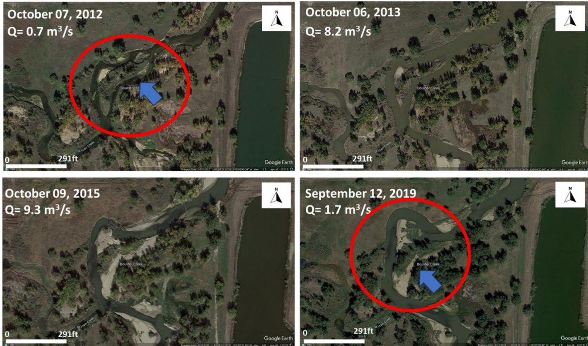
70 Figure 1: Change in channel width in Boulder Creek, Colorado, before (2012) and after (2013-2015-2019) a flash flood in 2013 (Google Earth imagery). The Discharge reported here is the daily discharge measured at USGS 06730200 Boulder Creek at north 75th St. near Boulder, co. The red circles denote the section of the channel that has changed over the years and the blue arrow shows the missing channel from the year 2012 to 2019.
