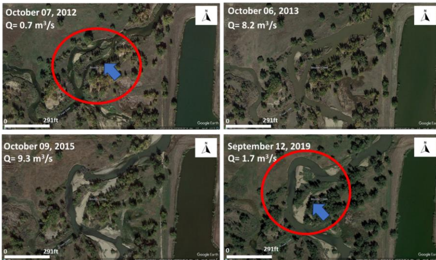
80 Figure 1: Change in channel width in Boulder Creek, Colorado, before (2012) and after (2013-2015-2019) a flash flood in 2013 (Google Earth imagery). The Discharge reported here is the daily discharge measured at USGS 06730200 Boulder Creek at north 75th St. near Boulder, co. The red circles denote the section of the channel that has changed over the years and the blue arrow shows the missing channel from the year 2012 to 2019.
