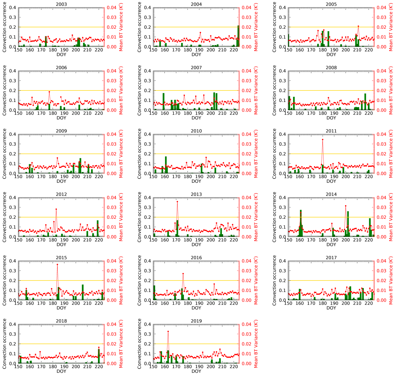
Figure A3. AIRS 8.1 \mu\text{m} deep convection (green bars) and 4.3 \mu\text{m} brightness temperature variances (red circles) averaged over the regions confined by the black and green boxes in Figure 2, respectively. The convection corresponds to the left axis and the brightness temperature variance corresponds to the right axis. The brown line shows the 0.02 \text{ K}^2 threshold chosen to highlight extreme gravity wave events.
