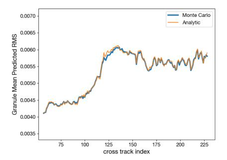
The RMS is lower in the regions of greater defocus, however the "L1 prediction" derived from the L1 radiance noise estimates also shows a similar trend - so this is likely related to the radiance pixel precision being better on that side of the detector.
