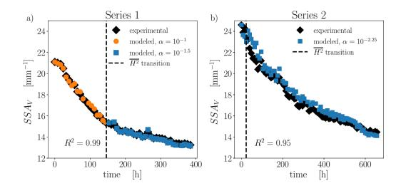
Figure 7. Comparison of experimental and modeled SSA time evolution. a) Series 1 with  $\alpha_{\text{Series1}}^{\text{best}}$  for  $t \le 160$  h and  $\alpha = 10^{-1.5}$  for t > 160h. b) Series 2 with  $\alpha_{\text{Series 2}}^{\text{best}}$ .
