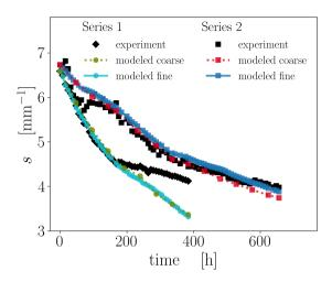
Figure 5. The time evolution of the SSA s for both series with coarse and fine temporal resolution for the best previously found values  $\alpha_{\text{Series 1}}^{\text{best}}$ ,  $\alpha_{\text{Series 2}}^{\text{best}}$ .
