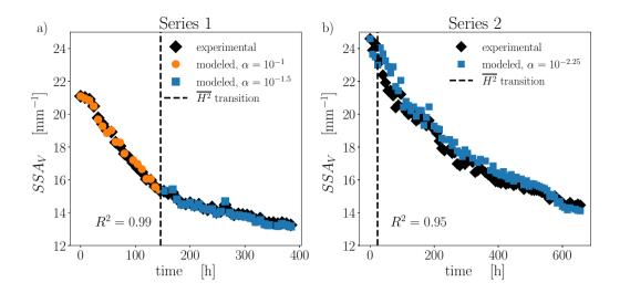
Figure 7. Comparison of experimental and modeled SSA time evolution. a) Series 1 with  $\alpha_{\text{Series 1}}^{\text{best}}$  for  $t \leq 160$  h and  $\alpha = 10^{-1.5}$  for t > 160 h. b) Series 2 with  $\alpha_{\text{Series 2}}^{\text{best}}$ .
