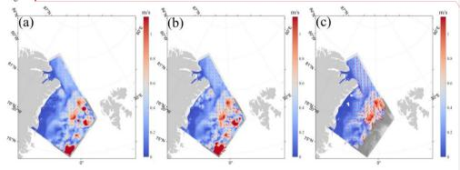
Figure 6: An example of quality control applied to <u>the retrieved SID</u>. (a: SID with no quality control, b: SID after neighborhood filter (only), c: SID after using neighborhood filter and cross-correlation value and its derived parameters filter).
