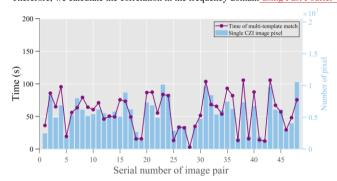
Figure 5: Relationship between multi-template matching time and image size.
