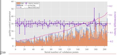
Figure 21: Relationship between the velocity difference and quality control parameters.
