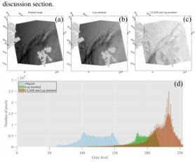
Figure 4: An example of <u>a</u> CZI image (<u>average of bands</u> 2, <u>3</u>, <u>and 4</u>) before and after data enhancement and <u>its grayscale histogram</u>.
