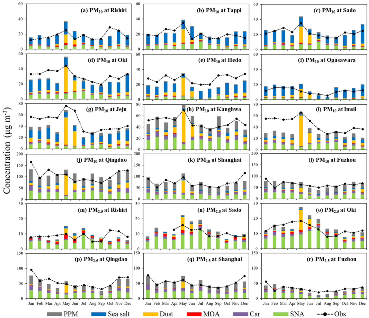
Figure 2. The model simulated (Sim) and observed (Obs) monthly PM_{10} (a~l) and PM_{2.5} (m~r) concentrations at EANET and CNEMC sites for the year 2014. The monthly data were averaged from hourly observations and the simulations were sampled according to the observations. Simulated aerosol components (PPM: primary anthropogenic PM, Sea salt, Dust, MOA, Car: anthropogenic BC+OC, SNA: sulfate+nitrate+ammonium) are also shown.
