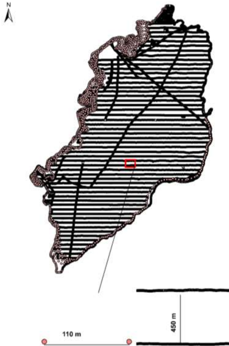
2 Figure 3: Bathymetry survey using multibeam echosounder (MBES) along predefined average 3 traverse lines at 450 m spacing along a north-south direction and 110 m along east-west 4 direction.
