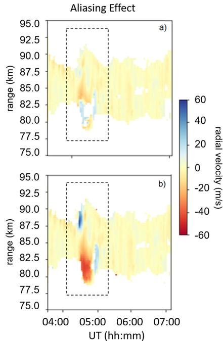
**Figure 3.** The colored contours show the vertical velocity (a) observed on July 16, 2016 after applying 6 additional coherent integrations (effective  $v_{\text{rad}} = 140$  m/s) and (b) without applying additional coherent integrations (effective  $v_{\text{rad}} = 175$  m/s) over altitude. The velocities cannot be determined from the spectra due to filtering and thus are missing in (a).
