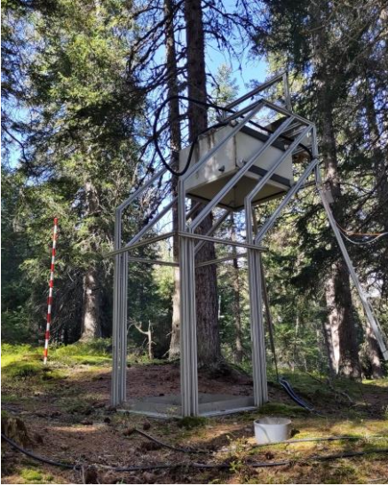
530 Fig. A.1: Picture of one of the automatic chambers (at location FF3).
