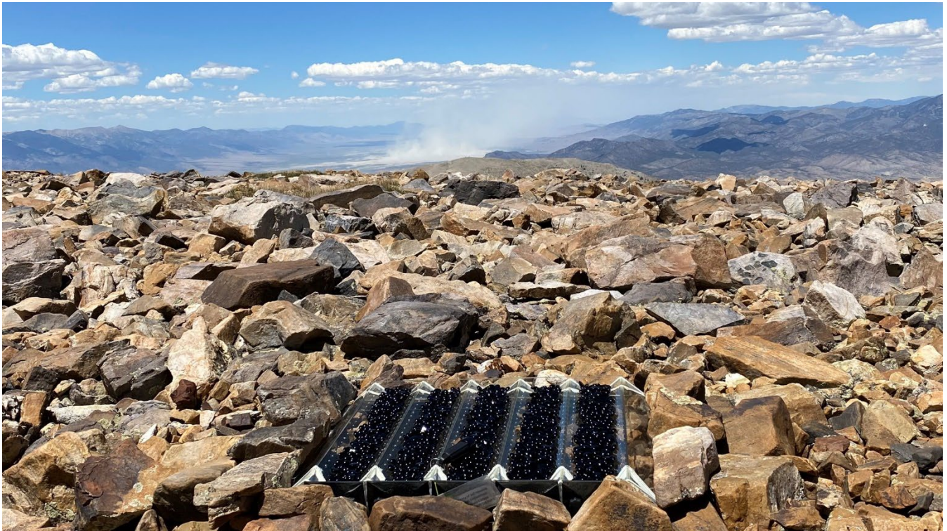
145 Figure 3. Photograph of the DUST-12 collector showing the sampler design (5 troughs with V-shaped cross sections filled with black, glass marbles), and the typical ground-level deployment. In the background a dust storm lifting material from the ground surface in the Spring Valley and transporting it to the east (right) into the North Snake Range is obvious.
