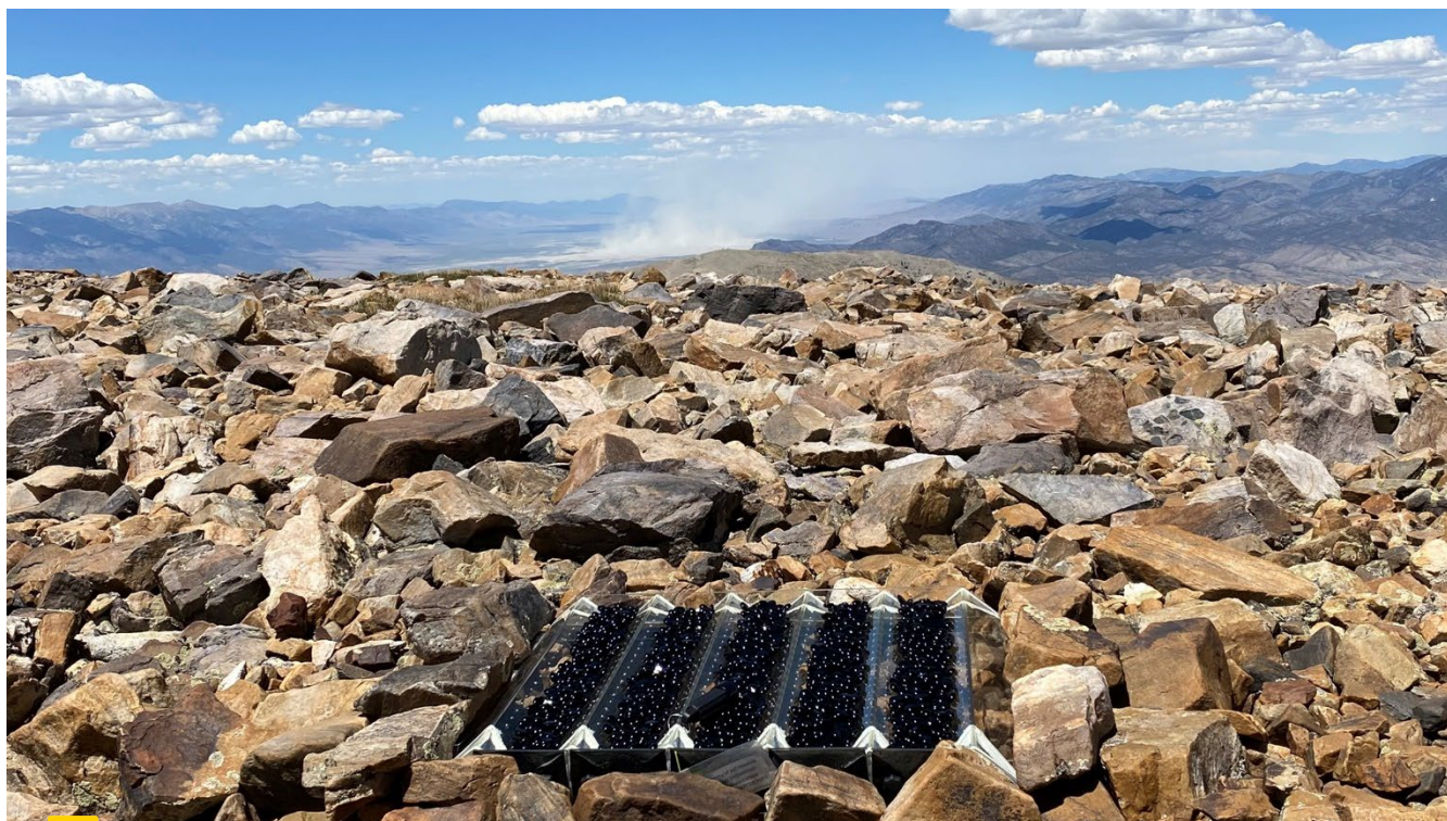
Fig. 1. Close-up photograph of the DUST-12 collector showing the sampler design (5 troughs with V-shaped cross sections filled with black, glass marbles), and the typical ground-level deployment. In the background a dust storm lifting material from the ground surface in the Spring Valley and transporting it to the east (right) into the North Snake Range is obvious.
