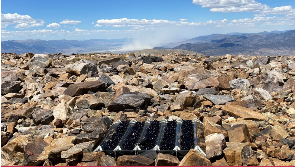
Figure 3. P Close-up photograph of the DUST-12 collector showing the sampler design (5 troughs with V-shaped cross sections filled with black, glass marbles), and the typical ground-level deployment. In the background a dust storm lifting material from the ground surface in the Spring Valley and transporting it to the east (right) into the North Snake Range is obvious.
