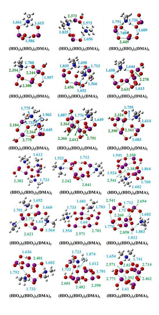
Figure 2. The most stable structures of HIO<sub>3</sub>-HIO<sub>2</sub>-DMA clusters identified at the ωB97X-D/6-311++G(3df,3pd) (for H, C, N and O atoms) + aug-cc-pVTZ-PP with ECP28MDF (for I atom) level of theory. The white, grey, blue, red, and purple balls represent the H, C, N, O, and I atoms, respectively. The hydrogen bonds and halogen bonds are shown in blue and green dashed lines, respectively. The values of bond lengths are given in Å.
