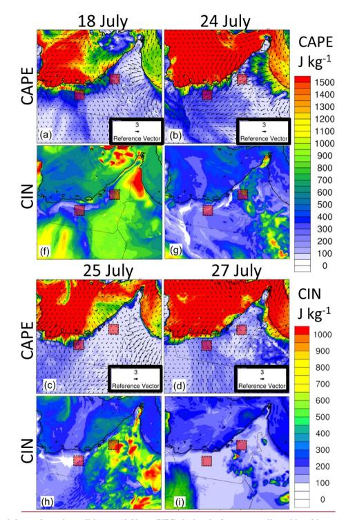
Figure 3: Control thermodynamic conditions at 10:00 am (UTC) during the four case studies, with red boxes to show the relative position of the ABS. The top row shows convective available potential energy (CAPE, J kg<sup>-1</sup>), 10<u>-</u>-m wind vectors, and a box showing
