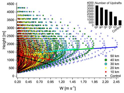
Figure <u>1412</u>: All vertical velocity values (0-4.5 km) and their heights on 27 July at 08:00 UTC within the 50 km footprint. A line of best fit for each scenario is also plotted to show the relationship of velocities with height. The bar chart shows the total number of updrafts for each scenario (within the 50 km zone) at 08:00 UTC.
