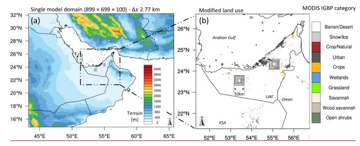
Figure 1: WRF model domain for all simulations, and the different scenarios used. Panel (a) shows the terrain over the northern Arabian Peninsula, and the inset model domain (2498 × 1942 km) centered on the United Arab Emirates (UAE) [dashed rectangle]. Panel (b) is the full extent of the model domain ( $\Delta x$  2779 m) showing MODIS IGBP land cover data. Also shown here are the five
