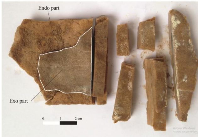
(c) preparation of sample SOY-19-02 for analyses. The white line indicates the limit between the endo and exo parts.
