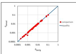
Figure 4. Plot of predicted values of near bed concentrations  $c_{bmod}$  using the modified formulation of Garcia and Parker (Equations 4a,b,c), versus those predicted from the original formulation,  $c_{borig}$  (Equations 1a,b,c). Calculation is conducted over the range of the Garcia-Parker data.
