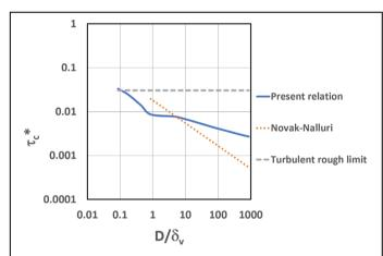
Figure A1. Critical Shields number  $\tau_c^*$  as a function of the ratio  $D/\delta_v$ , i.e. the ratio of grain size versus the nominal thickness of the viscous sublayer. Shown above are the relation for the limit of turbulent rough flow, the empirical relation of Novak and Nalluri (1975) for turbulent smooth flow, and the relation derived herein (present relation) for turbulent smooth flow.
