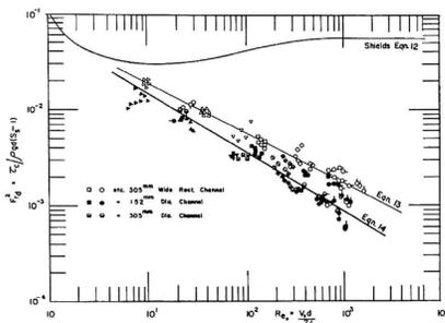
*Novak and Nalluri (1975) show the following diagram to the left, but do not discuss the reason as to why viscous effects reduce the critical Shields stress on a particle placed on a bed under turbulent smooth flow. They simply say: "Because of the mechanics of incipient motion, it is, of course, to be expected that in a conveyance with a fixed smooth bed the critical*
