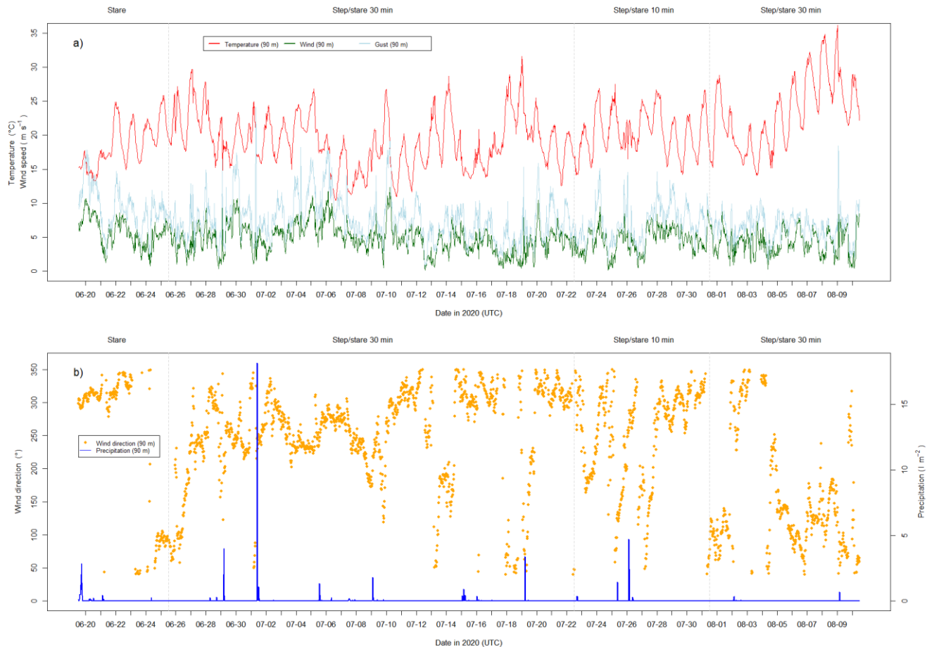
Figure 3: Overview over the meteorological conditions during the measurement period of 20 June 2020 – 10 August 2020 as measured by the sonic anemometer at a height of 90 m above ground on the lattice tower. We show temperature, wind speed, gust (a), and wind dire
