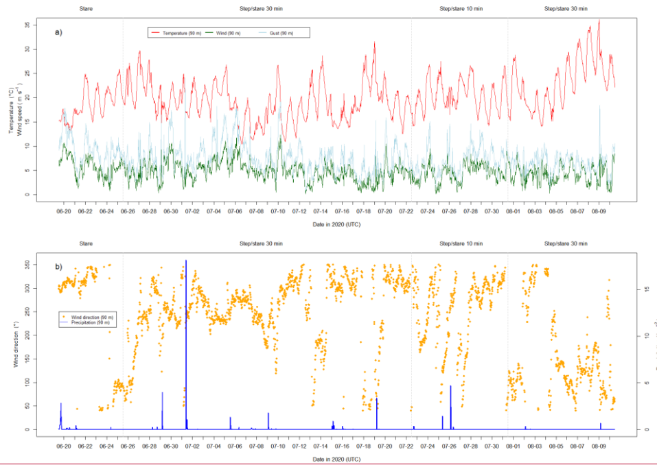
Figure 3: Overview over the meteorological conditions during the measurement period of 20 June 2020 – 10 August 2020 as measured by the sonic anemometer at a height of 90 m above ground on the lattice tower. We show temperature, wind speed, gust (a), and wind dire
