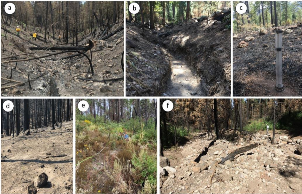
Figure 2: Examples of (a) the unchanneled valley bottoms that drained the lower portions of many watersheds prior to post-fire rainfall and a (b) gully incised during by post-fire rainstorms during-of the 2020 monsoon season. (c) A minidisk tension infiltrometer set up for a measurement at the mineral soil surface in an area with low soil burn severity. Note abundant needle cast and green canopy on trees in the background. (d) Canopy and ground cover were negligible shortly following the fire in July 2020 at the location of the moderate/high severity vegetation transect. (e) Understory canopy and litter cover substantially limited the fraction of bare ground at the moderate/high severity transect by September 2022. (f) Example of a debris flow deposit immediately upstream of Forest Road 3131A.
