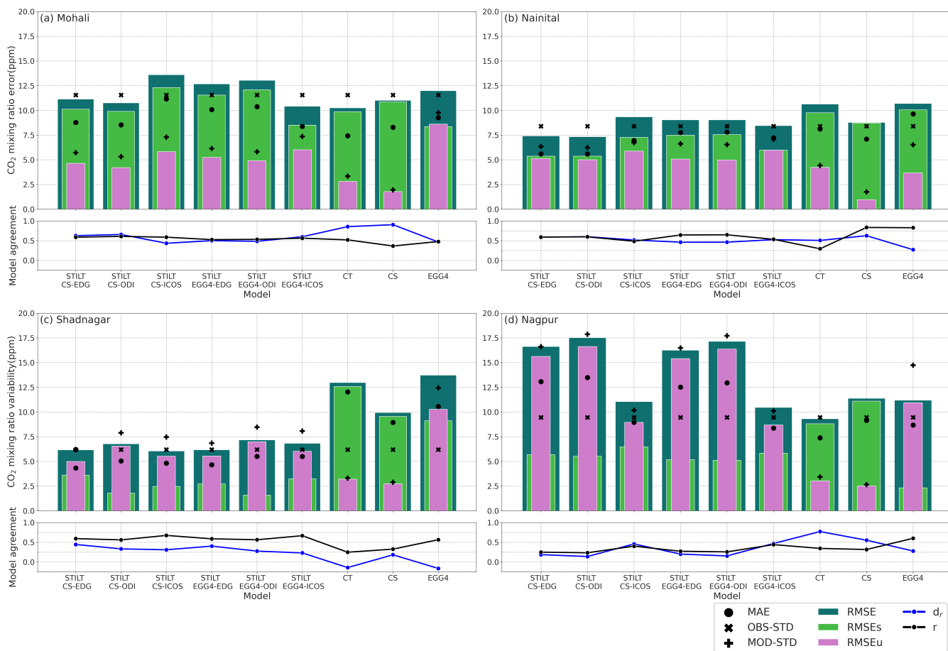
Figure 4. An overview of the performances of different models (see Sect. 4). Bar plots represent the different RMSE (in teal), systematic RMSE (RMSE s , in lime green) and unsystematic RMSE (RMSE u , in orchid) values estimated for each station. MAE (●), observed standard deviation (×) and model standard deviation (+) are overlaid on barplots. The blue and black lines represent the index of agreement (d r ) and correlation coefficient (r) values, respectively. The panels represent (a) Mohali, (b) Nainital, (c) Shadnagar, and (d) Nagpur stations.
