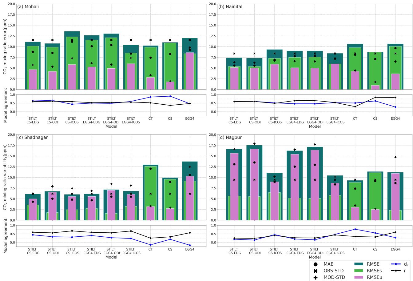
Figure 4. An overview of the performances of different models (see Sect. 4). Bar plots represent the different RMSE (in teal), systematic RMSE (RMSE s , in lime green) and unsystematic RMSE (RMSE u , in orchid) values estimated for each station. MAE (●), observed standard deviation (×) and model standard deviation (+) are overlaid on barplots. The black and blue and black lines represent the correlation coefficient and index of agreement (d r ) and correlation coefficient (r) values, respectively . The panels represent (a) Mohali, (b) Nainital, (c) Shadnagar, and (d) Nagpur stations.
