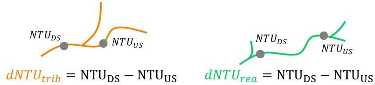
Figure 6. Differences in turbidity ( dNTU ) calculated as the upstream turbidity subtracted from the downstream turbidity. The locations of upstream and downstream turbidity are shown in the two panels: LEFT for tributaries and RIGHT for river reaches between two tributaries.
