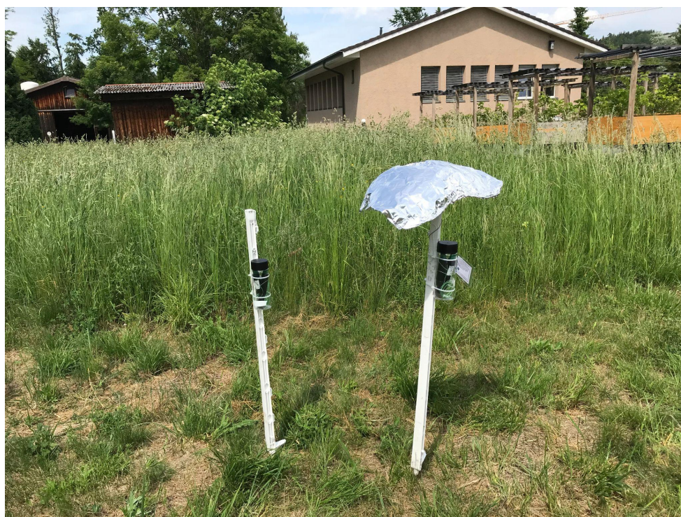
700 Figure E1: Example of shielding experiment with aluminium foil to determine if the logger measurements were affected by direct sunlight on the thermocouple. The thermocouple on the right pole was placed such that it was shaded throughout the day. The actual experiment consisted of a paired design, where we placed two shielded and two unshielded thermocouples in each of three representative environments for the field sampling (open, trees outside forests, and forest).
