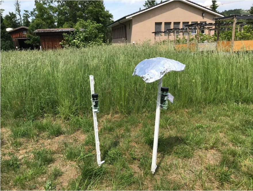
Figure F1: Example of shielding experiment with aluminium foil to determine if the logger measurements were affected by direct sunlight on the thermocouple. The thermocouple on the right pole was placed such that it was shaded throughout the day. The actual experiment consisted of a paired design, where we placed two shielded and two unshielded thermocouples in each of three representative environments for the field sampling (open, trees outside forests, and forest).
