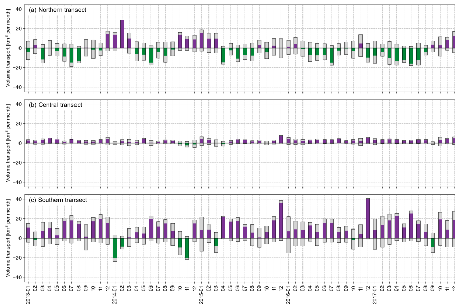
Figure 8. Monthly transport ( \text{km}^3 per month) in the whole water column lower layer in the northern (a), central (b), and southern (c) Archipelago Sea. Gray bars indicate the northward (positive) and southward (negative) monthly transport separately and the purple and green bars indicate the net transport. Note the different y axis limits compared to Fig. 7.
