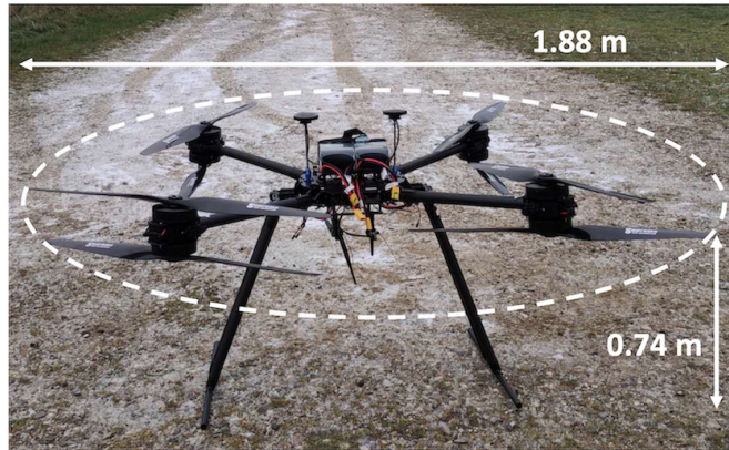
Figure 1. The Foxtech D130 x8, rotary-wing drone used in the experiment.
