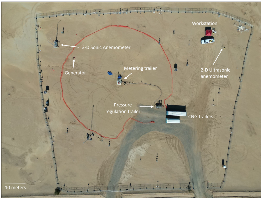
38 39 Figure 1. Aerial photograph of the site. Note that the workstation is ~60 m from the release apparatus and ~50m 40 from the compressed natural gas (CNG) trailers. Reproduced with permission from (El Abbadi et al., 2023).
