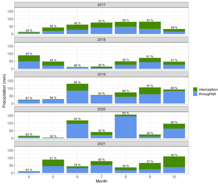
Figure : Local monthly precipitation, shown as stacked throughfall ( P_f mm) and interception ( P_i mm), at BIFoR FACE for treatment seasons 2017 to 2021. Percentage throughfall is indicated above each combined bar.
