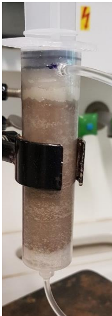
Figure S1.1: dry packed soil column
