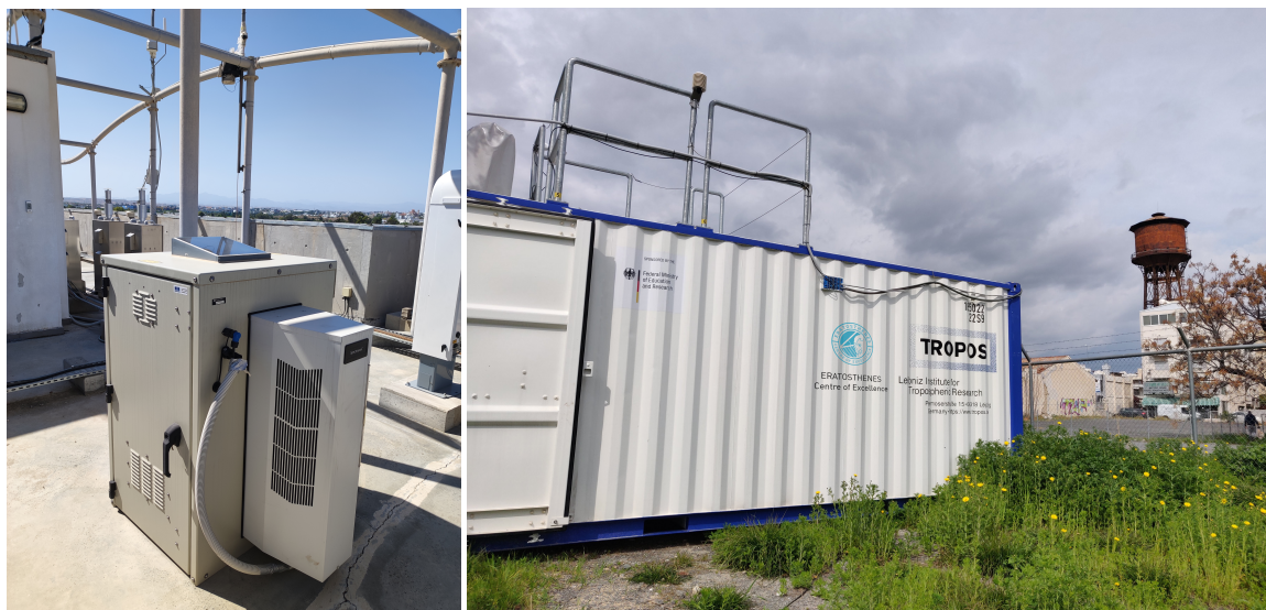
Figure 1. CE376 lidar with thermal enclosure on CYI premises roof in Nicosia (left) and Polly XT container housing in CUT premises in Limassol (right).
